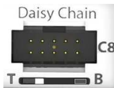
Figure 2-5. Terminator Resistor Switch (T) on Interface C8
