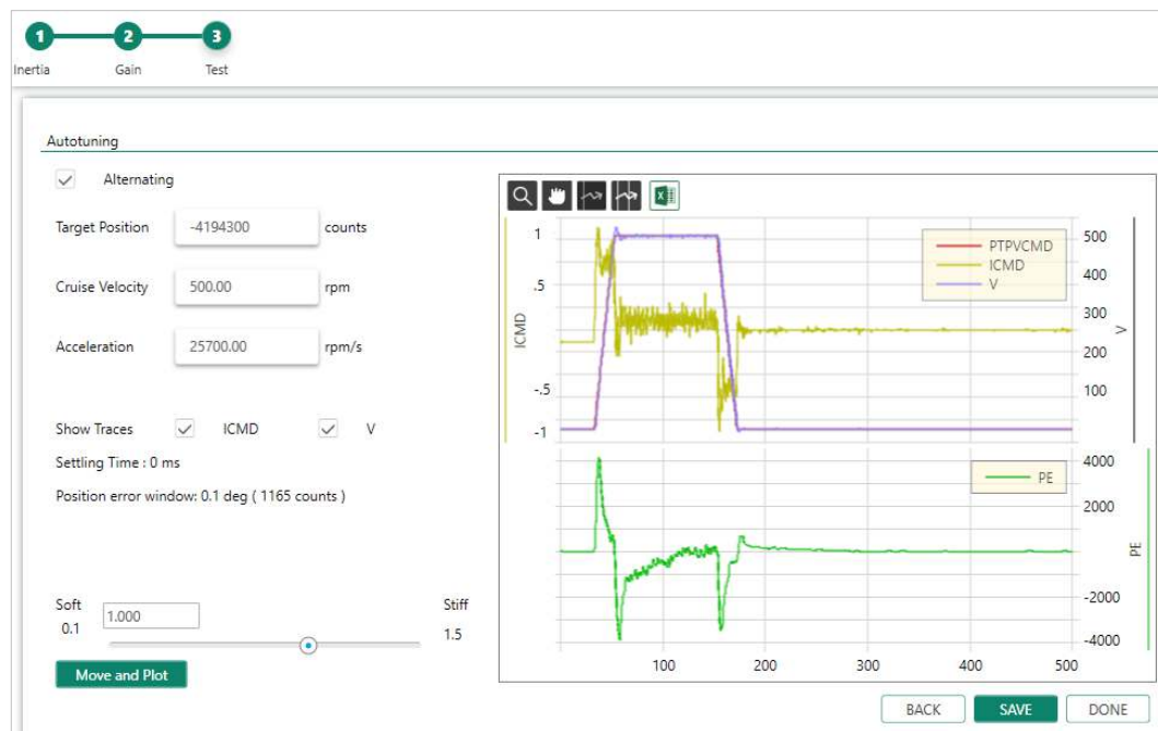
Figure 8-15. PC-Based Autotuning Wizard – Test Quality of Motion
