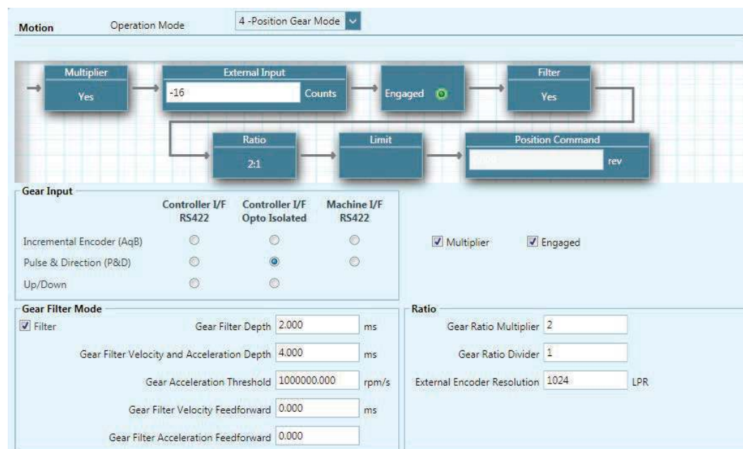
Figure 8-7. Motion Screen Settings for Pulse and Direction Commands Using a Single-Ended Signal
