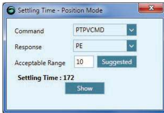
Figure 9-35. Settling time – with anti-vibration tuning
