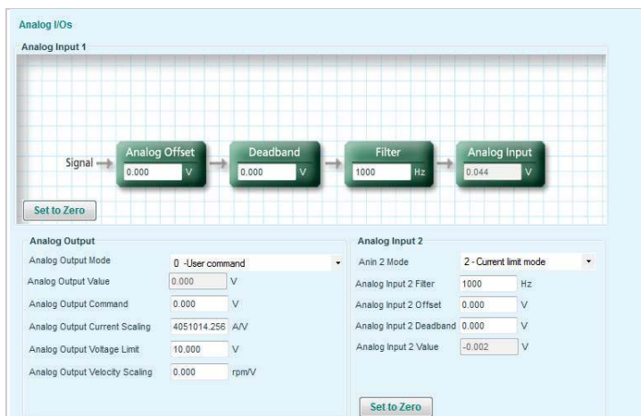
Figure 6-17. Analog Input 2 as Current Limiter
